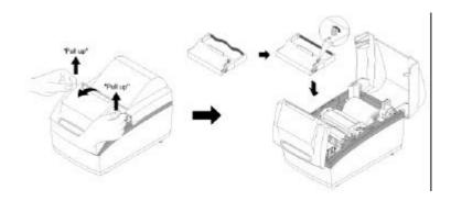
NOTE: Malfunctions and other problems may arise if other than the ribbon cassette samsung supplied is used. Samsung does not warrant against problems arising from the use of other than the ribbon cassette samsung supplied
